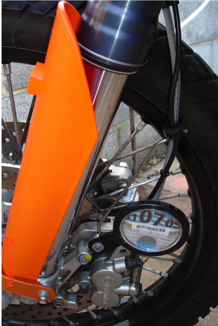
12. I've then made up my own protectors (the grey bits by the fender and by the fork legs) just to stop friction damage to the bits. I used pipe insulation foam wrapped in gaffer tape. Et voila! The finished job!
